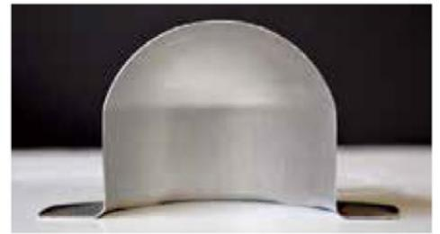
↑ A deep drawn part cross section shows uniform wall thickness. Because the material is wrapping around the punch tool as it is raised into the diaphragm, material is elongated more uniformly when compared to traditional drawing methods.
