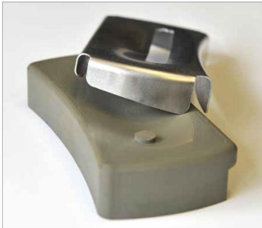
↑ This poured epoxy tool was a fast, economical option for this multi-bend part which features a stretch flange, a compression flange, and a return flange. Sheet hydroforming can replace press brake forming, consolidating multiple brake cycles into a single sheet hydroforming cycle.
