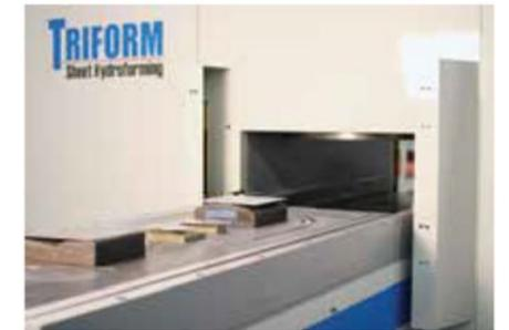
↑ A series of five different fluid cell tools rests unsecured on a sheet hydroforming press table. Benefits of the fluid cell sheet hydroforming process include the ability to run multiple different parts in a single press cycle.
