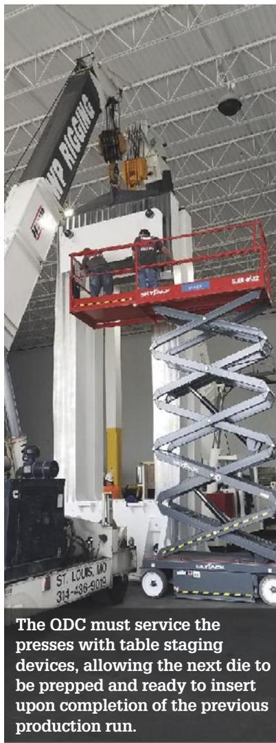
The QDC must service the presses with table staging devices, allowing the next die to be prepped and ready to insert upon completion of the previous production run.
