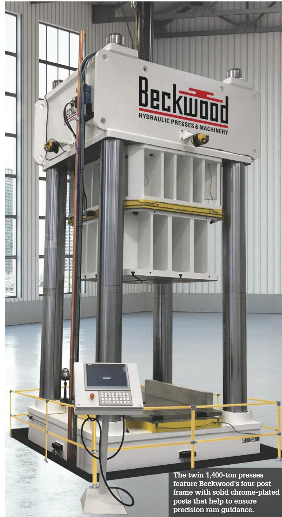
The twin 1,400-ton presses feature Beckwood’s four-post frame with solid chrome-plated posts that help to ensure precision ram guidance.
