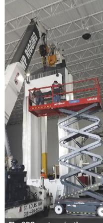
The QDC must service the presses with table staging devices, allowing the next die to be prepped and ready to insert upon completion of the previous production run.
