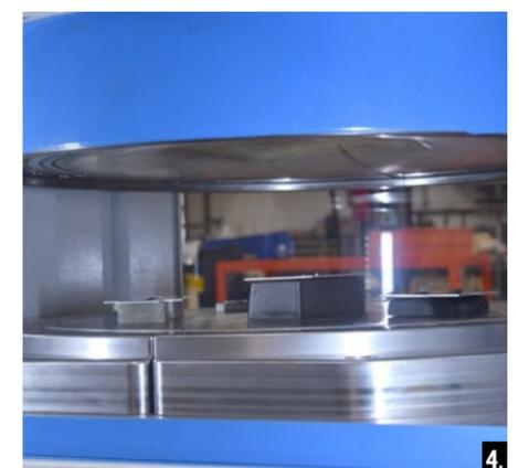
1. Deep-draw (top) compared to fluid-cell hydroforming (bottom). 2. Beckwood's Triform sheet hydroforming press installed at Jinpao Precision Industry Co. Ltd. 3. Checking a part produced on Beckwood's Triform sheet hydroforming press. 4. Sheet parts placed on tooling in preparation for hydroform pressing.
