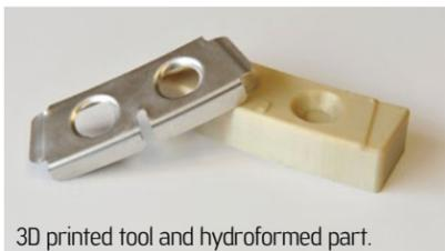
3D printed tool and hydroformed part.
