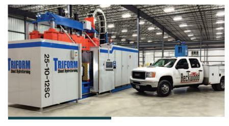
A Triform 25-10-12SC sheet hydroforming press. Beckwood offers its advanced PPM system on both its custom hydraulic presses, as well as on its Triform sheet hydroforming presses.
