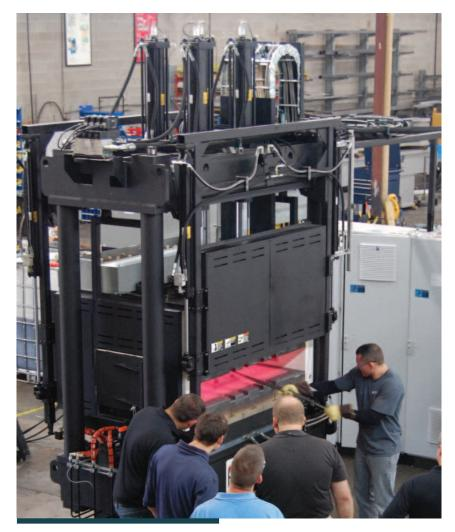
Beckwood's PPM system can be programmed to monitor and report when temperature variances are out of spec on heated platen presses.
