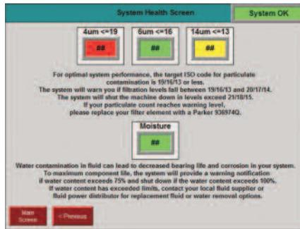
*This screenshot of the press’s fluid-health system helps operators understand how fluid contamination can impact press performance. The system provides warnings if fluid health declines past a defined point.*
